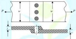
width of the plate w = 200 mm, thickness of the plate t = 5 mm, number of rivets n = 3, diameter of the rivet  $d_r = 10 \text{ mm}$ , diameter of the rivet hole  $d_b = 11 \text{ mm}$ , allowable tensile stress of the plate  $\sigma_p = 200 \text{ MPa}$ , allowable shear stress of the rivet  $\sigma_c = 150 \text{ MPa}$  and allowable bearing stress of the rivet  $\sigma_c = 150 \text{ MPa}$ .
