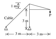
In the simple system shown in the figure, the load P is equal to 4 tonnes. What is the tension in the cable?
