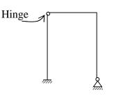
The kinematic indeterminacy of the frame is (a) 4 (b) 6 (c) 8 (d) 10 Ans: (c)
