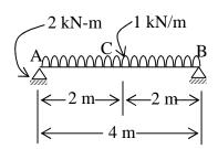
A freely supported beam AB of span 4 m is subjected to a UDL of 1 kN/m over the full span and a moment of 2 kN-m at support A as shown in the figure. The resulting BM at mid-span C of the beam will be
